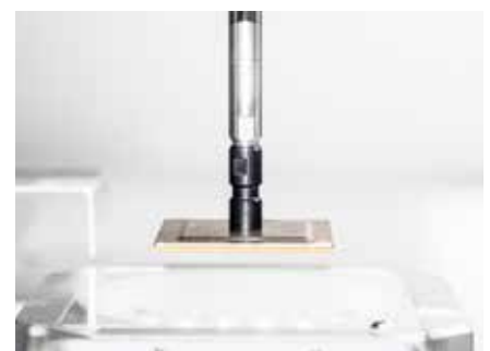
Metallic BGA above the light dome for detection of component connections
