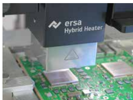
Homogeneous and reproduceable component heating thanks to the hybrid heating head
