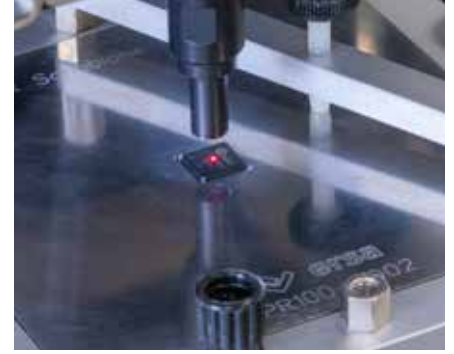
MLF component printed with solder paste is lifted out of a print stencil
