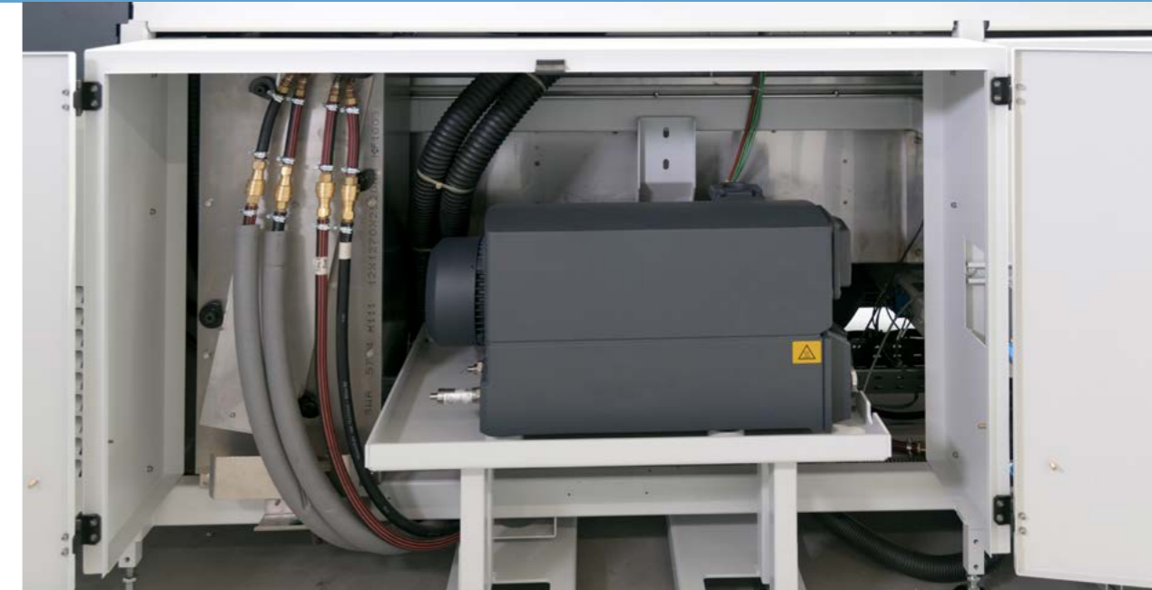
Vacuum unit semi-integrated in the back of the machine.
