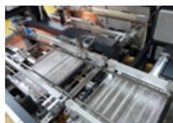
*In- and offline selective soldering system in a U-flow arrangement for modern manufacturing layouts*
