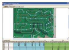
*Simple offline programming via DXF files or scanned PCBs with the ersa CAD Assistant provides for peak efficiency and machine uptime*
