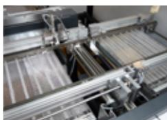
*Both short-wave IR emitters can optionally be upgraded with top-side convection heaters*
